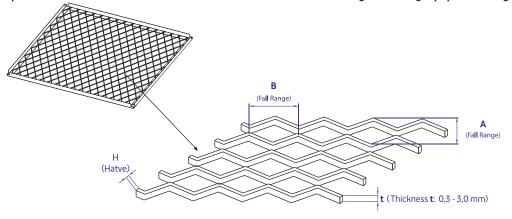
STANDARD MESH THICKNESSES and CELL SIZES (Thickness "t": 0.3 - 3.0 mm)
